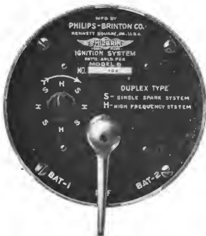
Left—Switch cover as it appears on cowboard. Right—Inside of switch showing the vibrator employed for the secondary ignition and the details of the selecting and reversing switch which gives either main or secondary ignition and-reverses the direction of the current with each click of the ratchet
